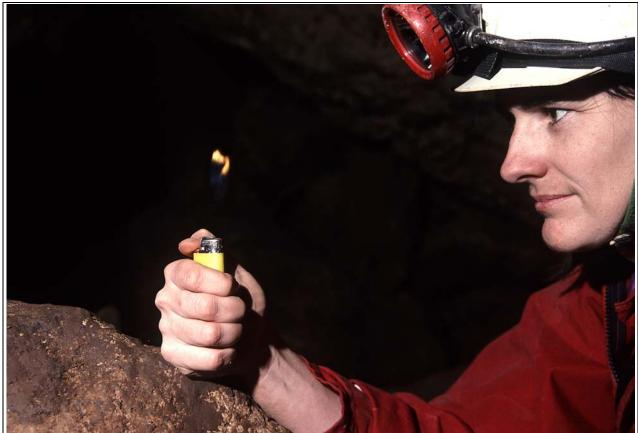
Jenny Whitby in Grill Cave, Bungonia NSW. Australia performs the flame test for foul air. The CO<sub>2</sub> on this occasion was measured at 5% with a Drager Meter. Photo by Garry K. Smith ©.
